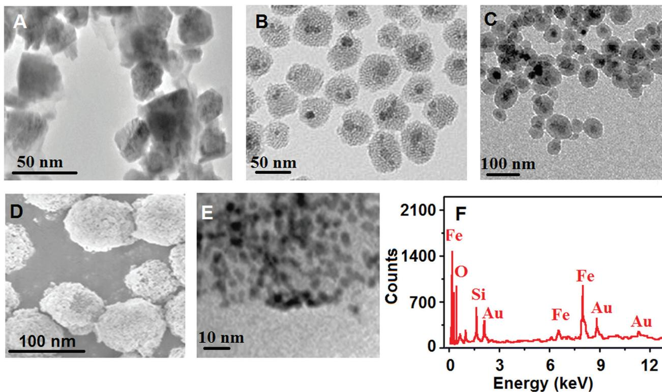
Fig. 3 TEM images of (A) Fe<sub>3</sub>O<sub>4</sub> NPs and (B and C) MMSNs, (D) SEM image of MMSNs@AuNPs, (E) HRTEM image of MMSNs@AuNPs, and (F) EDX spectra of MMSNs@AuNPs.
