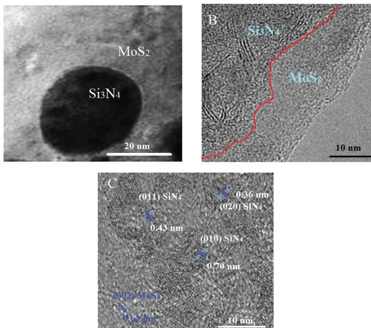
Fig. 2 TEM images (A–C) of the  $\text{Si}_3\text{N}_4/\text{MoS}_2$  composite.
