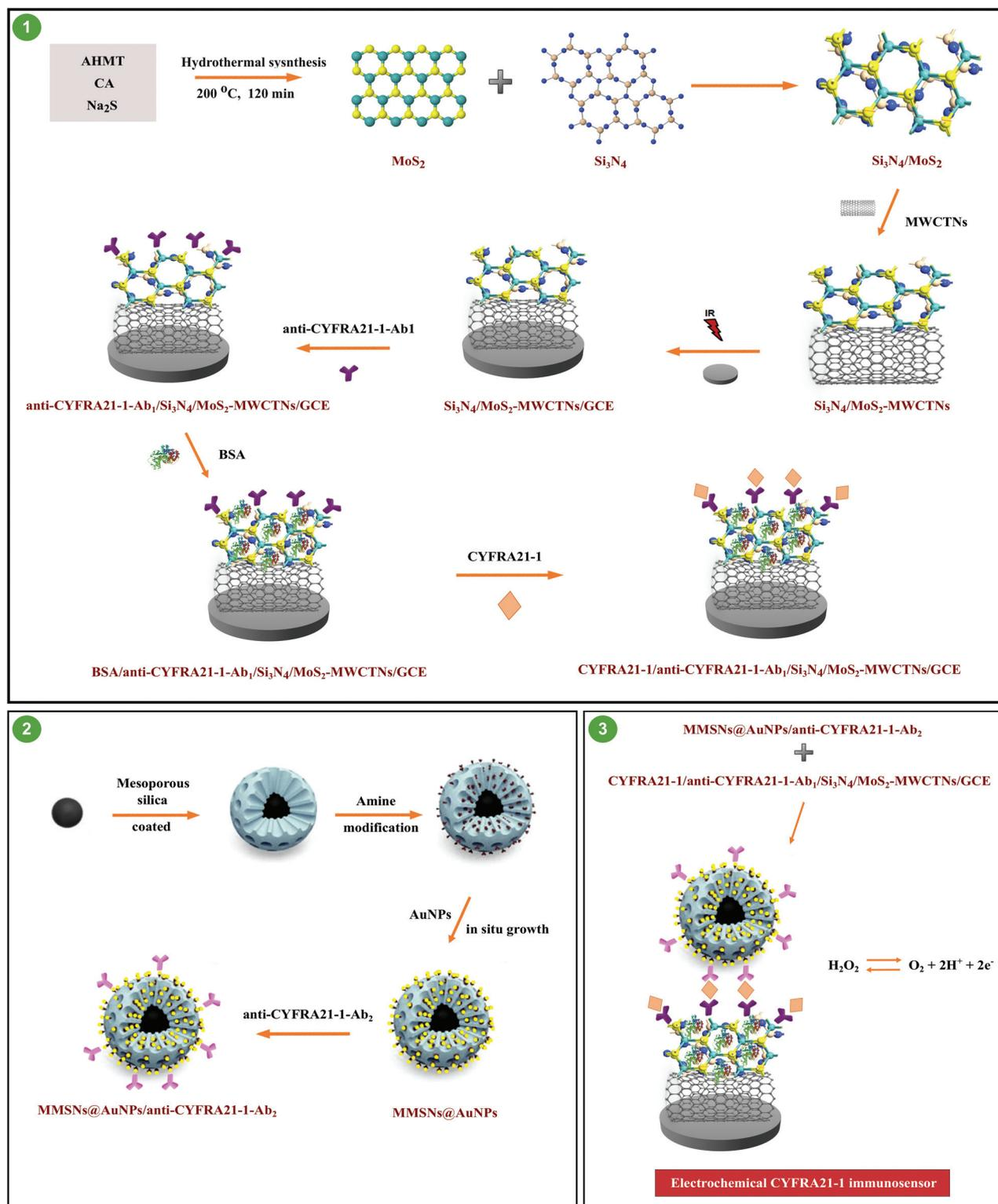
Scheme 1 Preparation procedure of the voltammetric CYFRA21-1 immunosensor.
