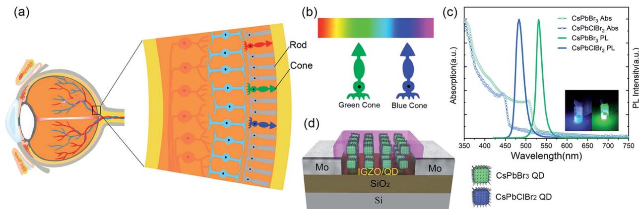
**Fig. 1** (a) The structure of the human eye retina. The color perception refers to the cones. (b) The absorption peaks of the blue and green cone cells in the human eye. (c) Absorption and photoluminescence (PL) spectra of CsPbClBr<sub>2</sub> QDs and CsPbBr<sub>3</sub> QDs. Inset: QD solutions under UV light. (d) Schematic diagram of a perovskite QD/IGZO phototransistor.
