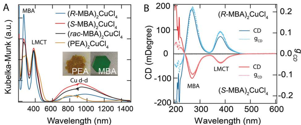
Fig. 12 (A) UV-vis-NIR spectra, and (B) CD spectra with the corresponding anisotropy factors of  $(R/S\text{-}rac\text{-MBA})_2\text{CuCl}_4$  and  $(\text{PEA})_2\text{CuCl}_4$ . Optical images of  $(\text{PEA})_2\text{CuCl}_4$  and  $(R\text{-MBA})_2\text{CuCl}_4$  crystals are shown in the inset. Reprinted with permission.<sup>104</sup> Copyright 2021, American Chemical Society.
