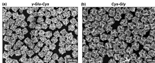
Fig. 7 (a) SEM images reveal crystal facets of chiral Au NPs generated by  $\gamma$ -Glu-Cys, and (b) Cys-Gly, respectively. Reprinted with permission.<sup>87</sup> Copyright 2020, Wiley-VCH.
