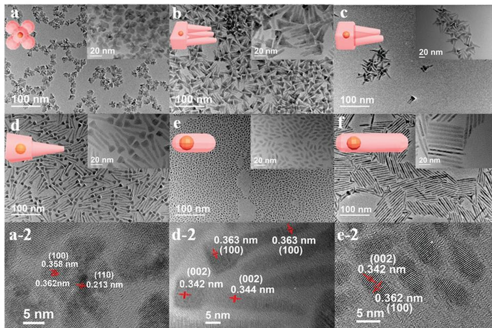
Fig. 9 (a–f) TEM images of CdSe/CdS NCs obtained in a variety of shapes including nanoflowers, Tadpole-III, Tadpole-II, Tadpole-I, short dot/rods, and long dot/rods. Reprinted with permission.<sup>91</sup> Copyright 2020, American Chemical Society.
