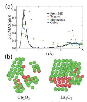
Fig. 3 (a) Comparative plot for partial  $Ce^{3+}-O^{2-}g(r)$  for our final  $Ce_2O_3$  nanoparticles obtained from molecular dynamics. The points indicated in the plot are the position and intensities for the pure infinite crystal in three different phases. (b) Visualization of low strain cations obtained for our final  $Ce_2O_3$  and  $La_2O_3$  models, using OVITO. The atoms shown as green are classified as cubic crystal atoms, while the red ones are trigonal.
