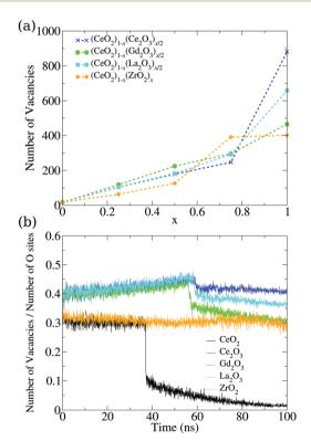
Fig. 7 (a) Dependency of the number of oxygen vacancies in the final structure on the relative concentration of the cations in mixed nanoparticles. (b) Evolution of the vacancy percentile in the oxygen sites of the pure structures. The total number of oxygen sites is also evolving, and is presented in Fig. S36 (ESI†).
