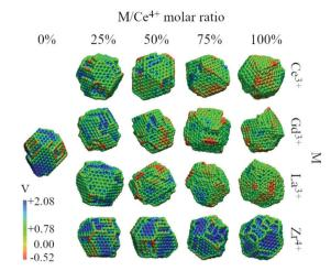
Fig. 10 Electrostatic potential map obtained with the particle-mesh Ewald method analysis for all nanoparticle structures at 0 K in relation to the M/Ce<sup>4+</sup> ratio
