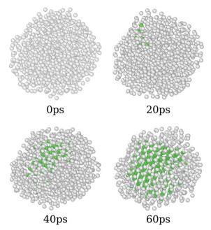
Fig. 4 Cations of the pure CeO<sub>2</sub> nanoparticle, colored by the neighborhood crystalline structure. Green atoms are located in the face-centered cubic sub-lattice sites, which are expected in the bulk fluorite CeO2 crystal, while white ones are in an amorphous or incomplete neighbourhood.
