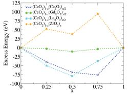
Fig. 6 Excess energy ( $E_{\rm exc}$ ) calculated from the structures at zero temparature.
