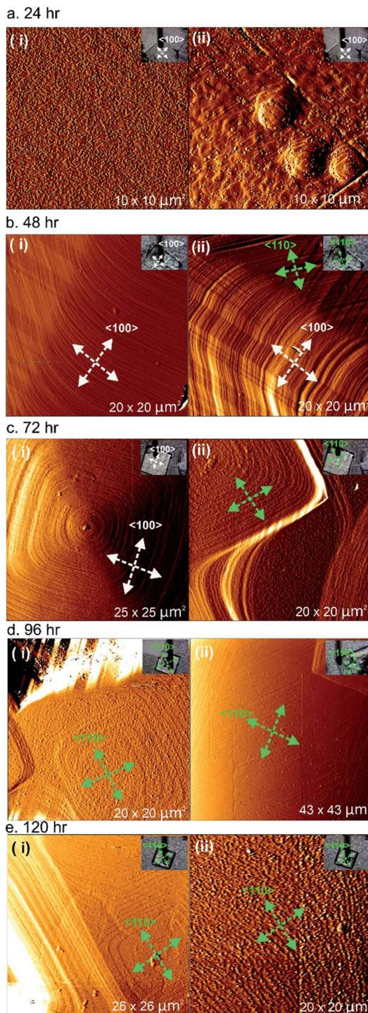
Fig. 2 *Ex situ* AFM deflection images of **1** formed after different reaction times. Optical images of the respective crystals of **1** are provided in the inset of each image. The white and green arrows indicate the  $\langle 100 \rangle$  and  $\langle 110 \rangle$  directions, respectively.
