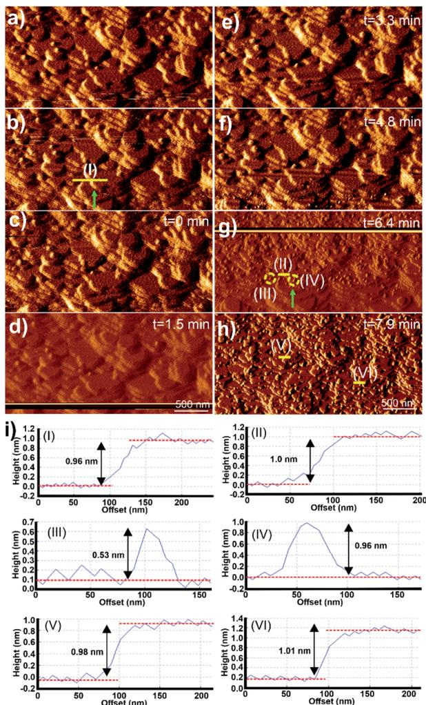
Fig. 4 A series of *in situ* AFM deflection images of **1** in the presence of DMF (a, b) and after the injection of the growth solution of **2** (c–h), and the corresponding cross-section analyses of selected terraces and 2D nuclei as indicated by yellow lines and circles respectively (i). AFM image sizes are  $3.0 \times 1.5 \mu\text{m}^2$ .
