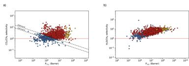
Fig. 4 Robeson trade-off plots for  $CO_2/CH_4$  (a) and  $H_2S/CH_4$  (b) ideal separations in 1685 MOFs. The  $CO_2/CH_4$  Robeson 1991 and 2008 limits are used to compare performance of each MOF to some of the best polymer membranes. 1183 MOFs lie above the 2008 limit (red and yellow points) and 35 (yellow points) are used in the study of binary mixture separations at working conditions of 10 bar and 298 K.
