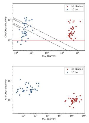
Fig. 5 Robeson trade-off plots comparing the  $CO_2/CH_4$  (top) and  $H_2S/CH_4$  (bottom) separation performance of 34 MOFs under infinite dilution (red) and at working conditions of 10 bar and 298 K (blue).
