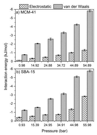
Fig. 10 The electrostatic and van der Waals interaction energy associated with the adsorption of  $CO_2$  molecules on the surfaces of MCM-41 and SBA-15 materials as a function of pressure are shown. These analyses are performed on data averaged over the last 10 ns of the simulation time. The error bars are calculated based on the simulations performed in triplicates.
