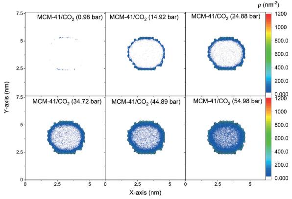
Fig. 5 The 2D density maps of the CO<sub>2</sub> molecules adsorbed on the pore walls of MCM-41 as a function of the pressure obtained from the classical molecular dynamics simulations are shown. The pore diameter of MCM-41 is 3.3 nm. The density maps are averaged over the last 10 ns of the simulation time.
