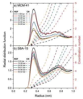
Fig. 8 The radial distribution functions and the corresponding coordination numbers of -OH-C<sub>CO</sub>, in the MCM-41 (a) and SBA-15 (b) as a function of the applied pressure are shown. The simulation data are averaged over the last 10 ns of the simulation time.
