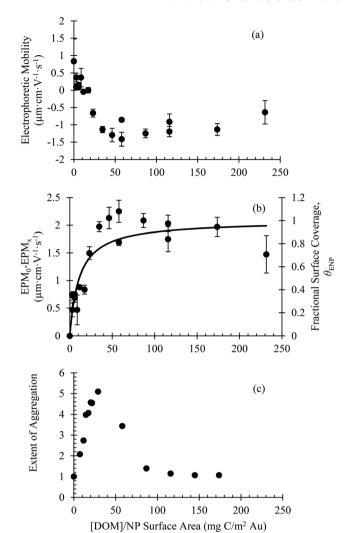
Fig. 2 (a) Electrophoretic mobility of bPEI-AuNPs (5 mg L<sup>-1</sup>); (b) change in electrophoretic mobility and fractional surface coverage  $(\theta_{\rm ENP})$  of bPEI-AuNPs (5 mg L<sup>-1</sup>); and (c) extent of homoaggregation of bPEI-AuNPs (2 mg L<sup>-1</sup>) in the presence of SRNOM. Error bars represent one standard deviation of replicates. Solution conditions included 1 mM HEPES, 20 mM NaCl and varying SRNOM concentrations.
