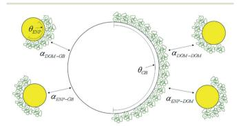
Fig. 1 Conceptual model for collisions between bPEI-AuNPs and glass beads in the presence of SRNOM.  $\alpha_{i-j}$  represent attachment efficiencies between surfaces of type i and j.  $\theta_{ENP}$  and  $\theta_{GB}$  represent the surface coverage of SRNOM on bPEI-AuNPs and glass beads, respectively.
