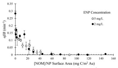
Fig. 4 Pseudo-first order rate constants ( $\alpha\beta B$ ) for attachment of bPEI-AuNPs (2 mg L<sup>-1</sup> or 5 mg L<sup>-1</sup>) to glass beads (20 g L<sup>-1</sup>) in 1 mM HEPES, 20 mM NaCl, and varying concentrations of SRNOM. Error bars represent one standard deviation of replicates.
