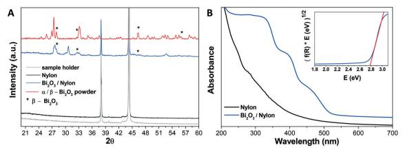
Fig. 2 A) XRD patterns of the sample holder, bare nylon, Bi<sub>2</sub>O<sub>3</sub>/nylon composite, and synthesized α/β-Bi<sub>2</sub>O<sub>3</sub> powder, and B) UV-vis DRS spectra of bare nylon and Bi<sub>2</sub>O<sub>3</sub>/nylon composite; inset: Tauc plot for the estimation of the bandgap.
