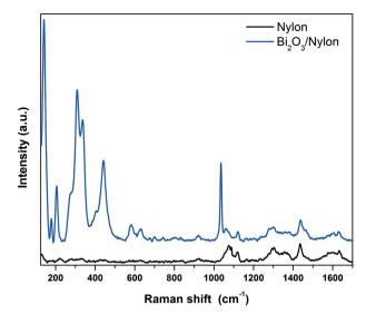
Fig. 5 Raman spectra of the bare (bottom black curve) and  $\alpha/\beta$ -Bi<sub>2</sub>O<sub>3</sub> decorated (top blue curve) nylon membranes.
