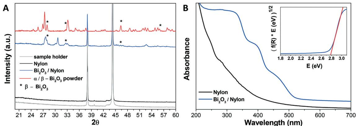
Fig. 2 A) XRD patterns of the sample holder, bare nylon, Bi<sub>2</sub>O<sub>3</sub>/nylon composite, and synthesized α/β-Bi<sub>2</sub>O<sub>3</sub> powder, and B) UV-vis DRS spectra of bare nylon and Bi<sub>2</sub>O<sub>3</sub>/nylon composite; inset: Tauc plot for the estimation of the bandgap.
