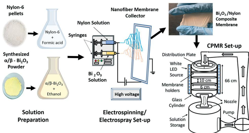
Fig. 1 Schematic layout of membrane preparation and photocatalytic tests.
