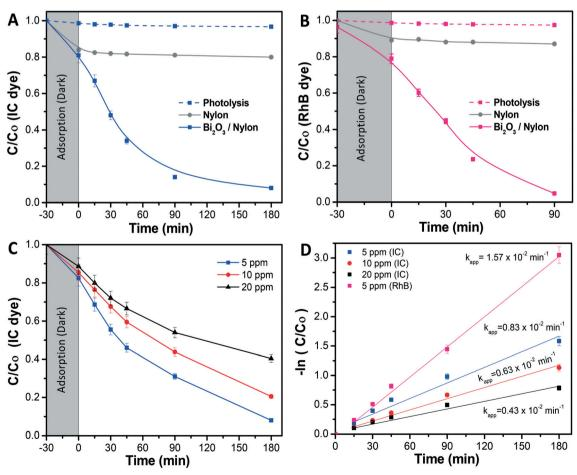
Fig. 6 Photocatalytic tests using bare nylon and Bi<sub>2</sub>O<sub>3</sub>/nylon composite membranes: A) relative concentration (C/C<sub>o</sub>) of IC degradation vs. time  $(C_o = 5 \text{ ppm})$ ; B)  $C/C_o$  of RhB degradation vs. time  $(C_o = 5 \text{ ppm})$ ; C)  $C/C_o$  of different IC dye concentrations with the  $Bi_2O_3/nylon$  composite membrane; and D) kinetic curve of IC and RhB dye solutions, and estimated apparent kinetic rates ( $K_{\rm app}$ ).
