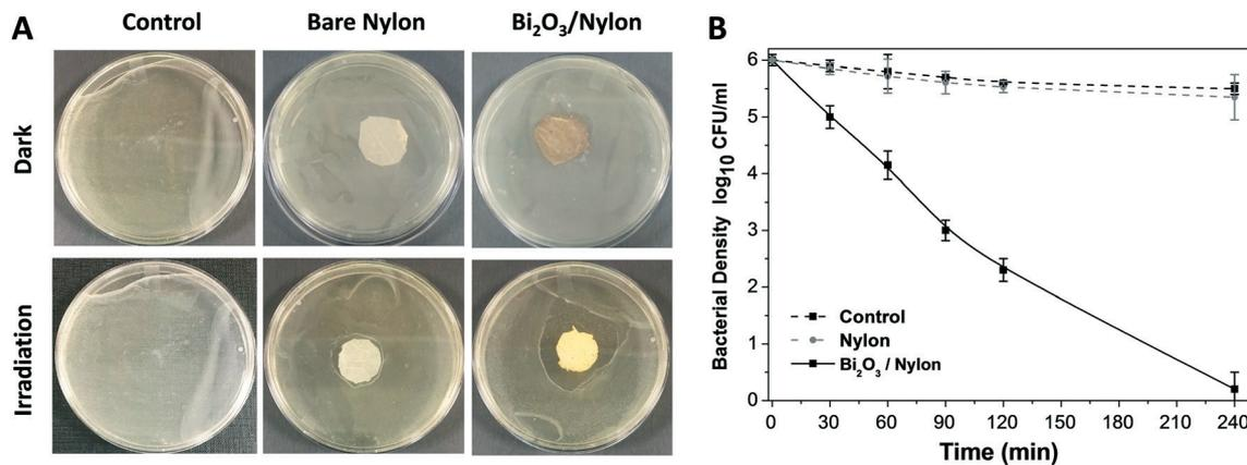
Fig. 8 A) Bacterial inhibition in solid media of control, bare nylon, and  $\text{Bi}_2\text{O}_3$ /nylon after incubation in the dark or under LED irradiation; B) *E. coli* density reduction in a liquid suspension treated with the photocatalytic  $\text{Bi}_2\text{O}_3$ /nylon membrane.
