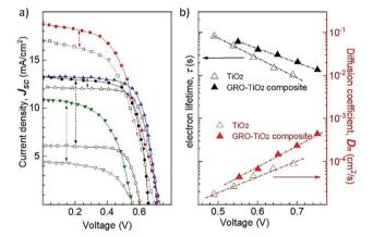
Fig. 14 (a) Typical J-V curves of DSSCs based on different GRM-based photoactive layers (line and full symbols) compared to those of the corresponding traditional TiO<sub>2</sub>-based photoelectrode. (b) Electron diffusion coefficient  $(D_n)$  and lifetime  $(\tau)$  dependence on the applied voltage for DSSCs based on TiO<sub>2</sub> photoactive layers with and without GRMs. Adapted from ref. 741,742,758,759.
