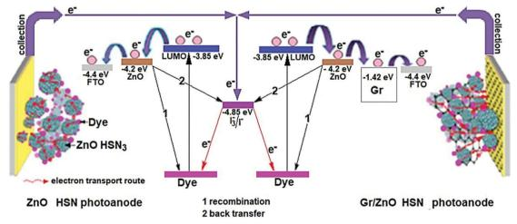
Fig. 12 Operating principle and energy diagram of the DSSC using ZnOHSN (left) or Gr/ZnOHSN (right.). Electron injection from the excited dye into the nanostructured ZnO semiconductor, electron transport to the collection electrode, and the recombination (1) and back transfer (2) pathways are also shown. Reprinted with permission from ref. 752, Copyright 2013, American Chemical Society
