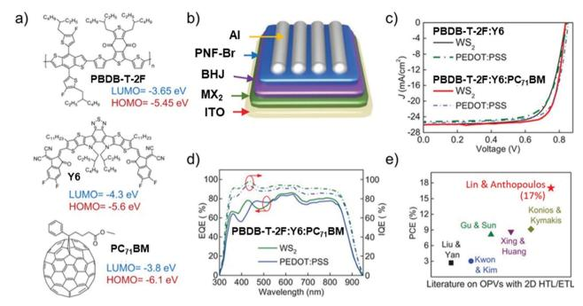
Fig. 10 (a) Chemical structure of PBDB-T-2F, Y6, and PC<sub>71</sub>BM and the corresponding LUMO and HOMO energies. (b) Schematic of the standard OSC architectures employed. (c) J-V curves of OSCs based on PBDB-T-2F:Y6 and PBDB-T-2F:Y6:PC<sub>71</sub>BM with different HTLs. (d) EQE curves of OSCs based on a PBDB-T-2F:Y6:PC71BM active layer for different HTLs. (e) A comparison of the performances of previously reported OSCs with 2D material interfaces. Adapted from ref. 633.
