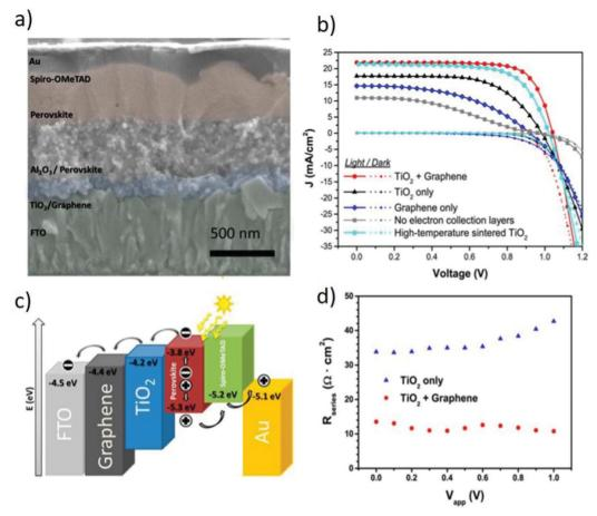
Fig. 19 (a) Cross-sectional SEM image of a PSC based on a graphene-TiO<sub>2</sub> composite as the ETL. (b) J-V curves measured for PSCs with different ETLs under solar irradiation and in the dark (c). Energy levels of a PSC based on a graphene-TiO2 composite as the ETL. (d) Series resistances of PSCs using pristine TiO2 and graphene-TiO2 composite as the ETLs. Reprinted with permission from ref. 1100, Copyright 2013, American Chemical Society.
