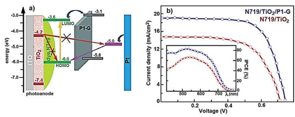
Fig. 13 (a) Schematic of the energy-level diagram and electron transfer process in P1-graphene-based DSSCs. (b) J-V curves and IPCE spectra for DSSCs with and without a P1-G layer. Adapted with data from ref. 769.
