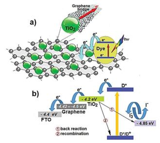
Fig. 11 (a) Schematic of light capture and electron transfer pathway from TiO<sub>2</sub> to the FTO, in TiO<sub>2</sub>/graphene-based DSSC photoanodes. (b) Schematic of the electron cascade route in DSSC using TiO<sub>2</sub>/graphene-based
