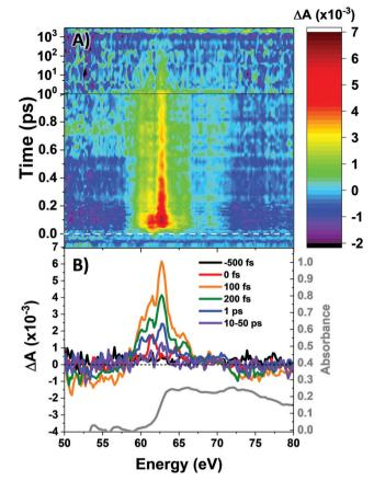
Fig. 2 (A) Contour plot of time-resolved M-edge XANES spectra. Time zero is indicated in the dashed white line. (B) Selected spectral slices with the ground state  $Co_4O_4$  spectrum in grey for comparison. The data are binned to 0.2 eV intervals
