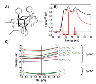
Fig. 1 (A) Structure of Co $_4$ O $_4$ . (B) Ground state M-edge XANES spectrum. The ligand field multiplet (LFM) simulation and sticks are shown in red. (C) Correlation diagram showing transitions between the  $3p_e3d_6$  ground state and  $3p_e3d_7$  core-hole excited state as a function of ligand-field strength 10Dq.
