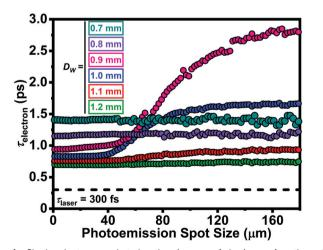
Fig. 4 Single-electron packet duration ( $\tau_{\rm electron}$ , fwhm) as a function of photoemission spot size for  $D_{\rm W}$  ranging 0.7–1.2 mm. The LaB<sub>6</sub>  $D_{\rm tip}$  was 180  $\mu m.$  The horizontal black dashed line ( $\tau_{\text{laser}}\!)$  represents the selected probe laser-pulse duration of 300 fs (fwhm). The  $h\nu$  = 4.81 eV distribution in Fig. 1d was used as the  $E_0$ .
