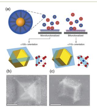
Fig. 8 (a) Scheme of DNA-functionalized nanoparticles assembled onto a DNA-functionalized substrate. (b and c) SEM images of  $\langle 100 \rangle$  or  $\langle 110 \rangle$  oriented crystals depending on the substrate functionalization. Scale bars, 1  $\mu m.^{67}$
