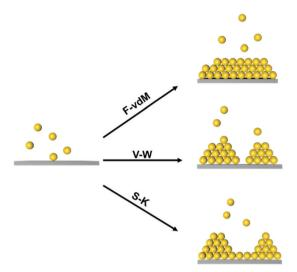
Fig. 1 Schematic illustration of three different modes in atomic epitaxial growth.
