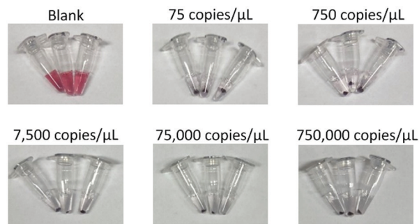
Fig. 3 Representative images from triplicate analysis of samples containing varying concentrations of the SARS-CoV-2 viral RNA. The N gene was detected. 5 μL of the viral RNA sample was used. The tubes labelled blank contained all reagents but no RNA sample (negative control).
