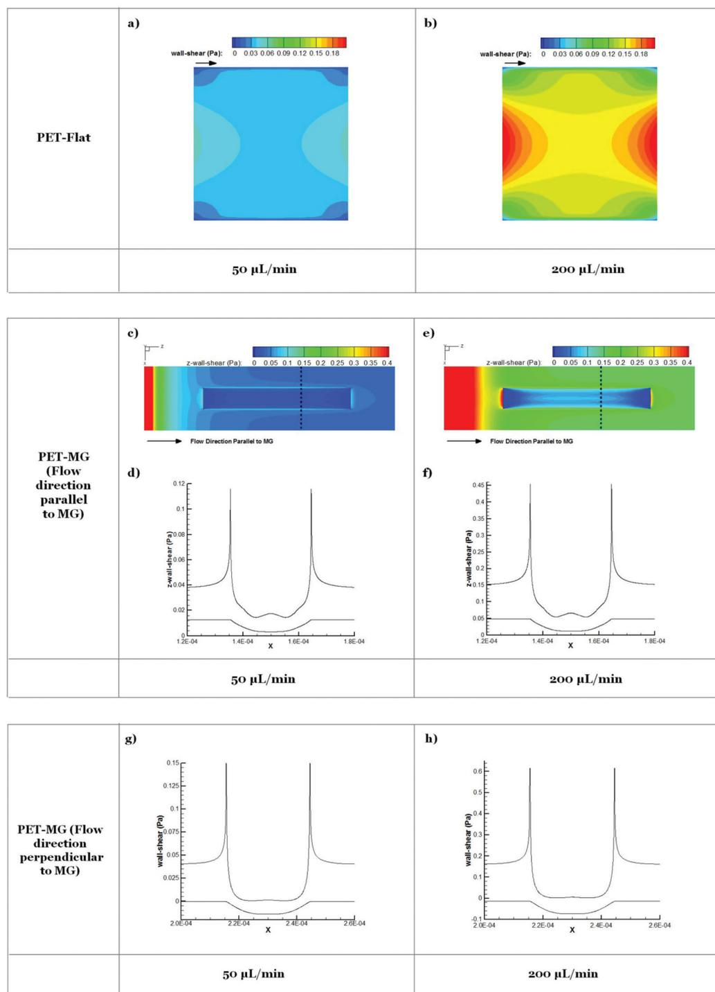
**Fig. 6** Contour plots on PET-Flat (a and b) and PET-MG substrates (c and e) and cross-section profiles (dotted line) (d, f, g and h) of computed wall shear stress for 50 (a, c, d and g) and 200  $\mu\text{L min}^{-1}$  (b, e, f and h) flow rates. Microgrooves are parallel (c–f) or perpendicular (g and h) to the flow direction. Lower curve in d, f, g and h depicts modeled geometry of microgroove cross-section.
