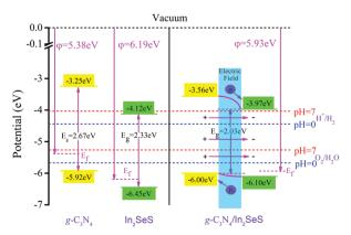
Fig. 6 Potential of band-edge positions for g-C<sub>3</sub>N<sub>4</sub>, monolayer In<sub>2</sub>SeS and the In<sub>2</sub>SeS/g-C<sub>3</sub>N<sub>4</sub> heterostructure.
