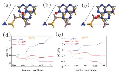
Fig. 10 (a)–(c) Optimized geometries of OH, O and OOH on the In<sub>2</sub>SeS/g-C<sub>3</sub>N<sub>4</sub> heterostructure during OER. (d) The changes of Gibbs free energy at pH = 0 and at different potential differences (0 V, 1.23 V and 1.56 V). (e) The changes of Gibbs free energy at pH = 7 and at different potential differences (0 V, 1.23 V and 1.97 V).
