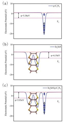
Fig. 5 (a) Electrostatic potential of g-C<sub>3</sub>N<sub>4</sub>. (b) Electrostatic potential of monolayer In<sub>2</sub>SeS. (c) Electrostatic potential of the In<sub>2</sub>SeS/g-C<sub>3</sub>N<sub>4</sub> heterostructure. The red and pink dashed lines denote the Fermi level and the vacuum energy level, respectively.
