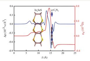
Fig. 2 Planar average charge density difference (blue line) and interfacial dipole moment (red line) along the Z-direction for the In<sub>2</sub>SeS/g-C<sub>3</sub>N<sub>4</sub> heterostructure
