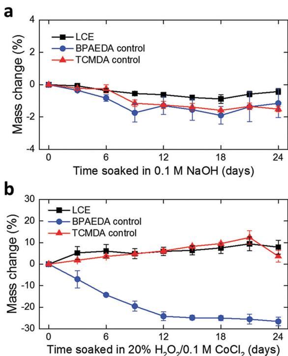
Fig. 2 Monitoring of mass change in LCE and control films over 24 days in (a) 0.1 M NaOH (mean  $\pm$  SD,  $n = 4$ ) and (b) 20% H<sub>2</sub>O<sub>2</sub>/0.1 M CoCl<sub>2</sub> (mean  $\pm$  SD,  $n = 4$ ), both at 37 °C.
