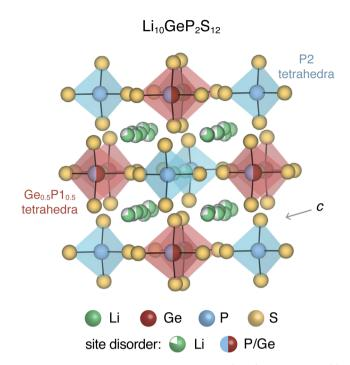
Fig. 1 Tetragonal crystal structure of Li<sub>10</sub>GeP<sub>2</sub>S<sub>12</sub> contains P2S<sub>4</sub> tetrahedra and (Ge<sub>0.5</sub>P1<sub>0.5</sub>)S<sub>4</sub> tetrahedra with partially occupied Li sites in the c-axis channels and in the a-b plane bridging sites. The S sublattice and P2 sites are fully occupied.
