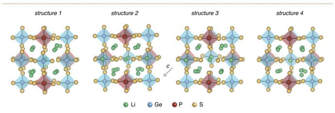
Fig. 3 Four representative LGPS structures selected for defect calculations. The structures differ in the Li site occupations and have slightly different volumes per atom (19.74, 19.84, 19.94, 20.02 Å<sup>3</sup> per atom).
