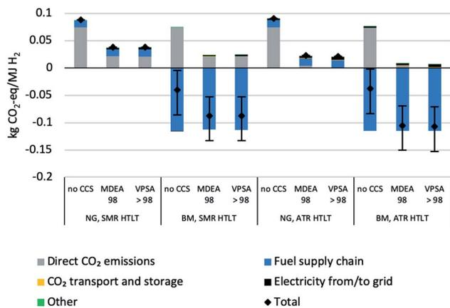
Fig. 6 Life cycle climate change impacts of H<sub>2</sub> production with natural gas (NG) or biomethane (BM) as feedstock/fuel, shown for the HT + LT configurations and 98% CO<sub>2</sub> capture rate in capture unit. Bars reflect the variations modelled in the cases presented in Scheme 9.
