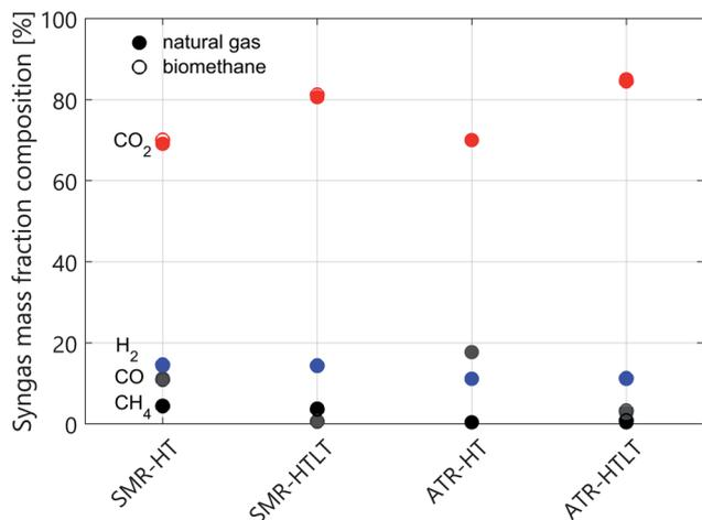
Fig. 1 Syngas composition of the four different hydrogen production pathways analysed. In red we show the  $\text{CO}_2$  mass fraction, in blue the one of  $\text{H}_2$ , in grey the one of  $\text{CO}$  and in black the one of methane. The full-dots represent the values obtained by reforming natural gas, while the empty circles represent the case with biomethane reforming.
