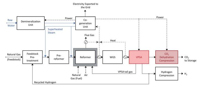
Scheme 5 Hydrogen production via steam methane reforming with VPSA CO<sub>2</sub> capture and H<sub>2</sub> purification. The VPSA unit replaces the PSA by integrating  $H_2$  purification and  $CO_2$  capture into a single separation unit. The recovered  $CO_2$  is then dehydrated and compressed, while the VPSA tail gas is burnt in the external furnace.
