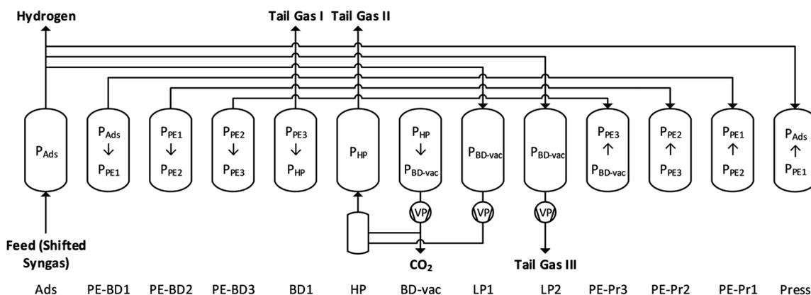
**Scheme 6** Schematic representation of the VPSA cycle for co-purification of CO<sub>2</sub> and H<sub>2</sub>. The cycle consists of 13 steps including a high pressure adsorption step during which H<sub>2</sub> is purified, an evacuation step during which high purity CO<sub>2</sub> is withdrawn, and several recycle and purge steps. Tail gas is produced as third outlet stream.
