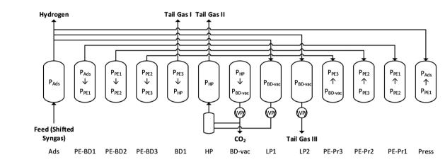
Scheme 6 Schematic representation of the VPSA cycle for co-purification of CO<sub>2</sub> and H<sub>2</sub>. The cycle consists of 13 steps including a high pressure adsorption step during which H2 is purified, an evacuation step during which high purity CO2 is withdrawn, and several recycle and purge steps. Tail gas is produced as third outlet stream.
