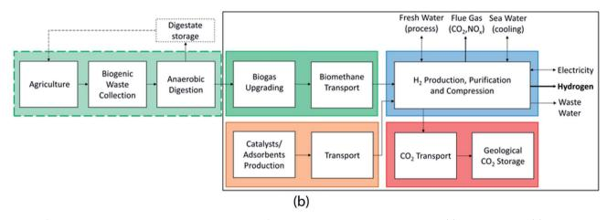
Scheme 7 System boundaries and allocation choices for the LCA of  $H_2$  production based on natural gas (a) and biomethane (b) with and without CCS.
