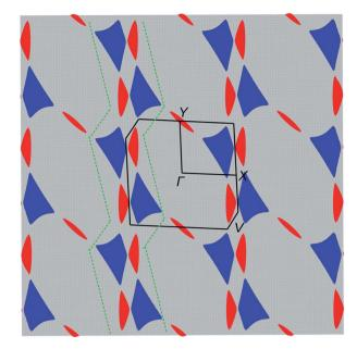
Fig. 6 DFT calculations. Fermi surface of BO4 in an extended Brillouin zone, which is composed of electron (blue) and hole (red) pockets associated with the ( $\Gamma$ , X and Y) symmetry points in the bands. Black lines represent the first Brillouin zone, and green dotted lines represent the hidden 1D Fermi surface.
