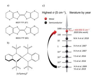
Fig. 1 Organic conductors and single-molecule magnets. (a) Structural diagrams of BEDT-TTF (ET) and BEDO-TTF (BO). (b) Tetrahedrally coordinated structure of [Co(pdms)<sub>2</sub>]<sup>2-</sup>. (c) The evolution of the highest  $\sigma$  by year for the reported conducting SMM materials: black and red dots represent semiconductors and metals, respectively. The original literature abbreviated in this panel is listed in ref. 12.
