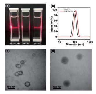
Fig. 2 (a) Tyndall effect seen for PtC<sub>10</sub> ⊂ CP6A aggregates prepared in aqueous solutions of different pH. (b) DLS data for PtC<sub>10</sub> ⊂ CP6A and DOX@PtC<sub>10</sub> $\subset$ CP6A (298 K, scattering angle = 90°). TEM images: vesicles self-assembled from (c) PtC<sub>10</sub> ⊂ CP6A and DOX@PtC<sub>10</sub>  $\subset$  CP6A ([CP6A] = 0.05 mM and [PtC<sub>10</sub>] = 0.10 mM).
