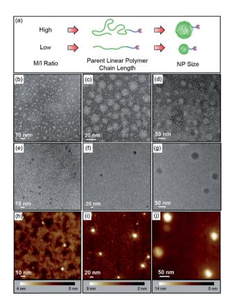
Fig. 3 (a) Illustration of the synthesis of different-sized monovalent  $ONP-N_3$ . (b-d) Negatively stained TEM images of  $ONP^{S/M/L}$ . (e-g) Brightfield TEM images of  $ONP^{S/M/L}$  using ultrathin carbon layer grid. (h-j) AFM images of  $ONP^{S/M/L}$  using PeakForce Tapping mode under ambient condition.
