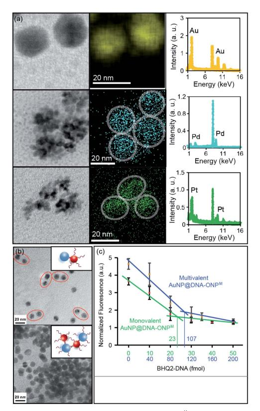
Fig. 6 (a) STEM and EDX element mapping of AuNP, PdNP and PtNP synthesized from ONP<sup>M</sup>. (b) Hybridization-mediated MNP dimerization using the AuNP@DNA-ONPM and commercial AuNP functionalized with complementary DNA strands. (c) Fluorescence titration plots of monoand multivalent AuNP@DNA-ONP<sup>M</sup>. Note: the fluorescence intensity of the multivalent AuNP was normalized. Its actual fluorescence intensity was much stronger than the monovalent AuNP.
