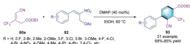
Scheme 24 DMAP-catalyzed [4 + 2] benzannulation to synthesize penta-substituted benzenes.
