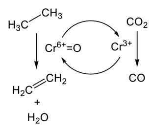
Scheme 1 Redox mechanism for EDH in the presence of  $CO_2$  over Cr oxide catalysts.
