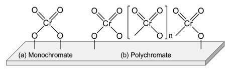
Fig. 8 Structure of (a) monochromate and (b) polychromate supported on a metal oxide.
