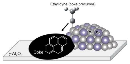
Fig. 7 Schematic image of the drain-off mechanism. Coke precursors such as ethylidyne move to the supports on which coke formation
