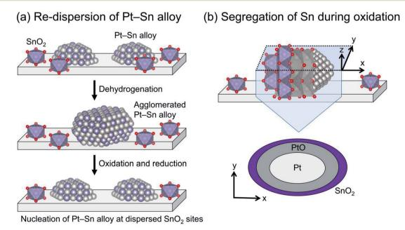
Fig. 5 Schematic images of (a) re-dispersion of Pt-Sn alloy through oxidation and subsequent reduction (regeneration) and (b) segregation of Sn from Pt-Sn alloy during oxidation.
