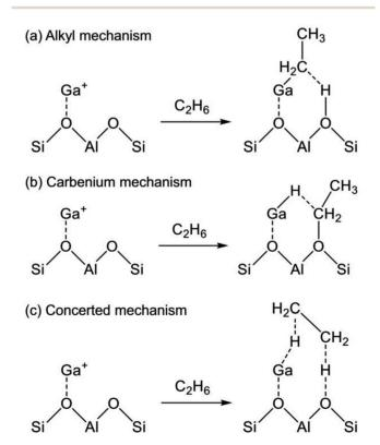
Scheme 2 Mechanism of ethane activation *via* (a) the alkyl mechanism, (b) the carbenium mechanism, and (c) the concerted mechanism. Ga<sup>+</sup> is a representative active site of Ga/H-ZSM-5.
