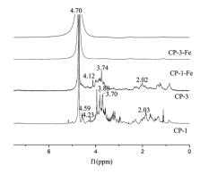
Fig. 5 <sup>1</sup>H NMR spectra of polysaccharides and polysaccharide-iron(III) chelates.
