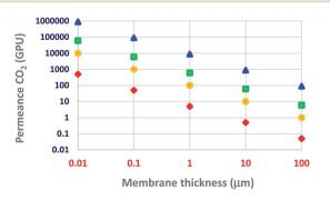
Fig. 3  $CO_2$  permeance as a function of membrane thickness: triangle, PIM-1; square, 6FDA-DAM; circle, Pebax® 1657; rhombus, polysulfone.<sup>29,41–43</sup>
