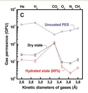
Fig. 7 Gas transport behavior of ultrathin GO membranes prepared by Kim  $et\ al.^{90}$
