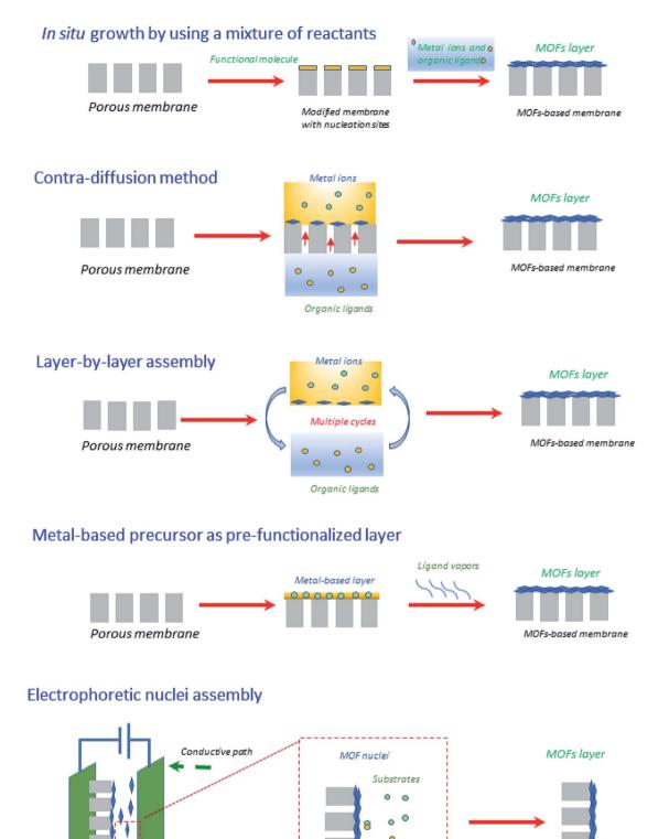
Fig. 5 Graphical illustration of different strategies for creating ultrathin MOFs-based membranes.<sup>44</sup>
