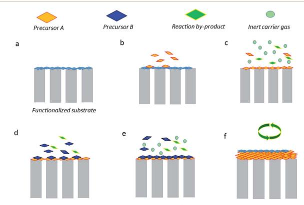
Fig. 6 Graphical illustration of the most common stages of the ALD technique.<sup>65</sup> (a) Functionalized support. (b) Precursor A reacts with the surface. (c) Purge of A and by-products. (d) Precursor B reacts with the surface. (e) Purge. (f) Repetition of (b-e) steps to achieve the target film thickness.
