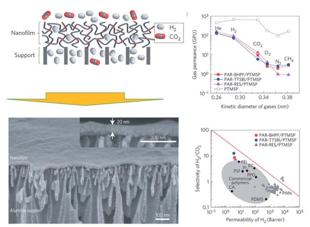
Fig. 8 Interfacial polymerization of polyacrylate-based nanofilms and their gas separation performance. Adapted from Jimenez-Solomon *et al.*99
