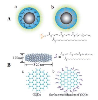
**Fig. 3** (A) Depiction of C-dots (a) following the treatment of surface oxidative and (b) following functionalizing with the surface-passivation reagent. (B) (a) A schema of the GQDs and (b) structural patterns following the functionalization with the surface-passivation reagents. Reprinted with permission. Copyright 2006, American Chemical Society.
