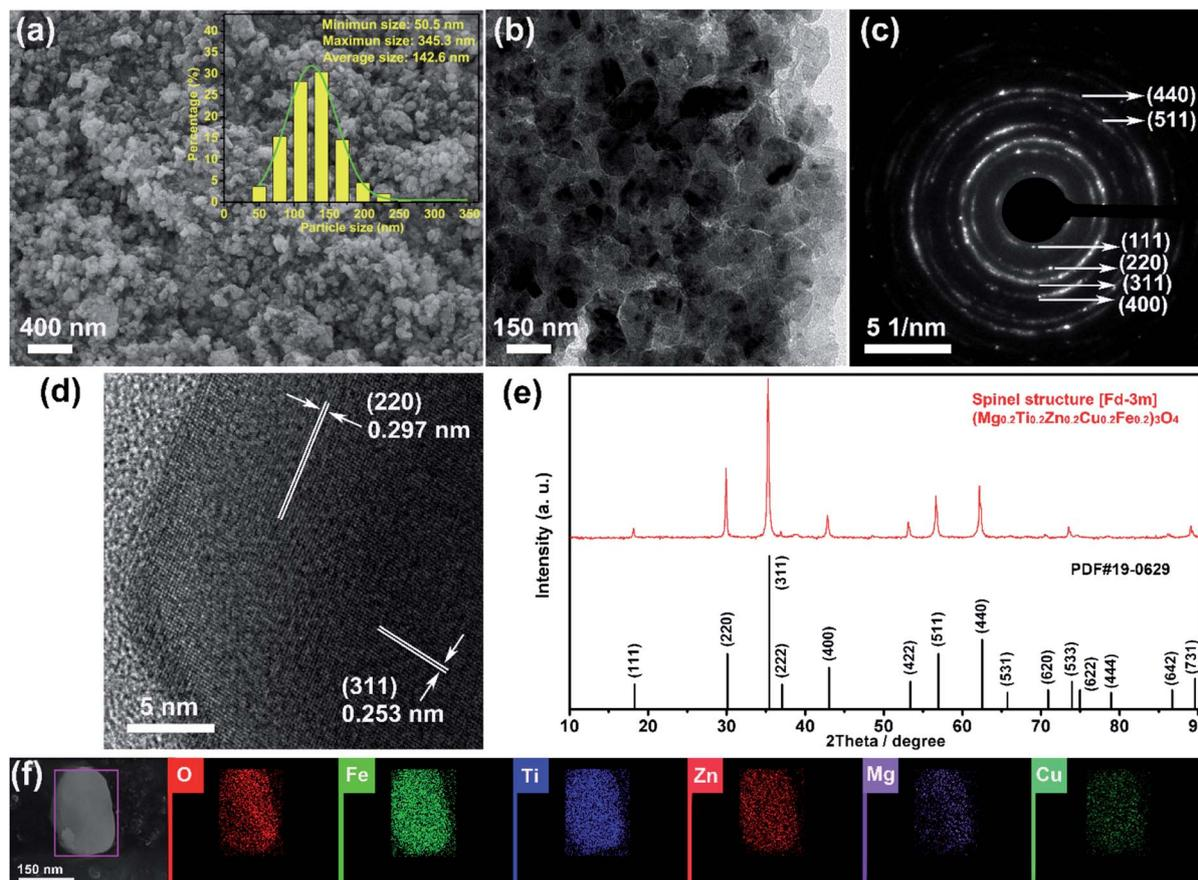
Fig. 1 (a) SEM image and (b) TEM image of the synthesized irregular  $(\text{Mg}_{0.2}\text{Ti}_{0.2}\text{Zn}_{0.2}\text{Cu}_{0.2}\text{Fe}_{0.2})_3\text{O}_4$  particles; (c) SAED pattern, (d) HR-TEM image, (e) XRD pattern and (f) elemental mapping images of the  $(\text{Mg}_{0.2}\text{Ti}_{0.2}\text{Zn}_{0.2}\text{Cu}_{0.2}\text{Fe}_{0.2})_3\text{O}_4$  particles.
