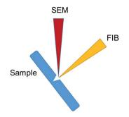
Fig. 9 Schematic showing the positioning of the sample, FIB and SEM beams during FIB-SEM cross sectioning.
