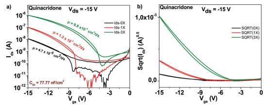
Fig. 9 (a) Comparison of OFET devices with three different purity grades of quinacridone semiconductor: unpurified  $(0 \times \text{in graph legend})$ , one time purified (1× in graph legend) and three times purified, respectively (3× in graph legend); (b) the  $sqrt(I_{ds})$  vs.  $V_{qs}$  of the three purity grades presented in panel (a).
