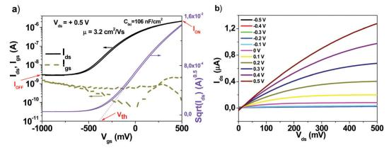
Fig. 3 (a) Transfer and (b) output characteristics of an organic field effect transistor which was part of the same batch as the one presented in ref. 60, as Fig. 4(c and d). Adapted with permission from ref. 60, G. Schwabegger, et al., High Mobility, Low Voltage Operating C<sub>60</sub> based n-type Organic Field Effect Transistors, Synth. Met., 2011, 161, 2058-2062.
