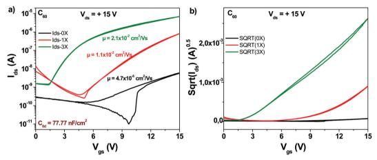
Fig. 5 (a) Comparison of OFET devices with three different grades of fullerene ( $C_{60}$ ) semiconductor purity: unpurified ( $0 \times$  in graph legend), one time purified (1× in graph legend) and three times purified respectively (3× in graph legend); (b) the  $sqrt(I_{ds})$  vs.  $V_{as}$  of the three purity grades presented in panel (a).
