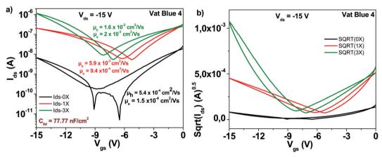
Fig. 8 (a) Comparison of OFET devices with three different purity grades of vat blue 4 semiconductor: unpurified (0× in graph legend), one time purified  $(1 \times \text{in graph legend})$  and three times purified, respectively  $(3 \times \text{in graph legend})$ ; (b) the sqrt( $I_{ds}$ ) vs.  $V_{qs}$  of the three purity grades presented in panel (a).
