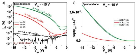
Fig. 10 (a) Comparison of OFET devices with three different purity grades of epindolidione semiconductor: unpurified ( $0 \times$  in graph legend), one time purified (1× in graph legend) and three times purified, respectively (3× in graph legend); (b) the  $sqrt(I_{ds})$  vs.  $V_{as}$  of the three purity grades presented in
