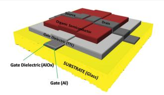
Fig. 2 OFET device architecture in the bottom gate-top contact configuration.
