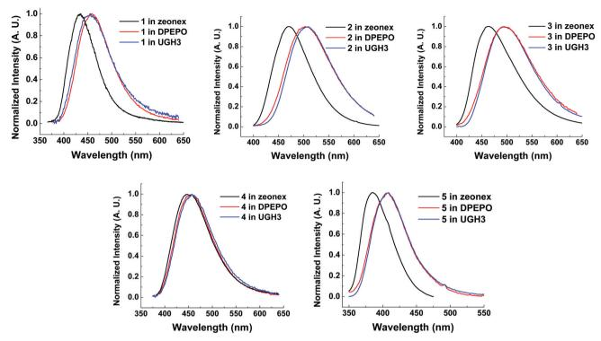
Fig. 6 Normalized steady state emission spectra from drop cast films of molecules 1–5 at 10 wt% in solid state hosts at room temperature.  $\lambda_{\rm exc}$  = 355 nm.
