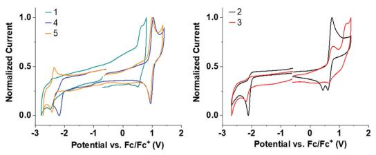
Normalized CV redox curves for 1-5 in deoxygenated MeCN solvent. All curves are referenced to the Fc/Fc<sup>+</sup> redox couple.
