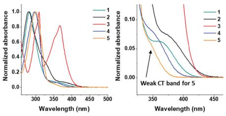
Fig. 4 Normalized absorption spectra for molecules 1-5 in DCM solution at 25  $\mu$ M (left) and 75  $\mu$ M (right). The weak shoulder attributed to the direct CT absorbance band in 5 is indicated. Higher concentration was used to obtain accurate measurement for onset of CT absorption band. Negligible red-shift in this band between the two concentrations was observed
