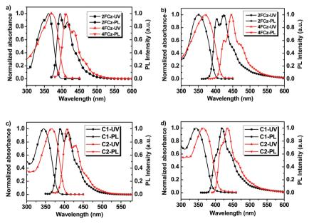
Fig. 3 UV-Vis absorption and PL spectra of (a) xFCz in solution, (b) xFCz in neat films, (c) Cx in solution, and (d) Cx in neat films.
