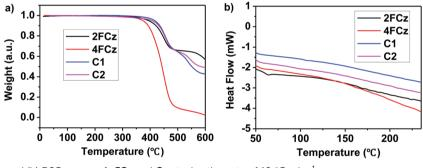
Fig. 1 (a) TGA thermograms and (b) DSC curves of xFCz and Cx at a heating rate of 10 °C min<sup>-1</sup>
