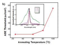
Fig. 7 Evolution of the ASE threshold as a function of annealing temperature for (a) C1 and (b) C2; insert: normalized ASE spectra from r.t. to 200 °C.
