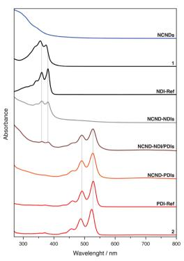
Fig. 4 UV-Vis absorption spectra of rylene diimide precursors (1 and 2), references (NCNDs, NDI-Ref, PDI-Ref) and hybrid materials (NCND-NDIs, NCND-PDIs, NCND-NDI/PDIs) in DMF, at room temperature. Vertical lines in grey are guides to help the comparison between the naphthalene and perylene diimide-based materials.
