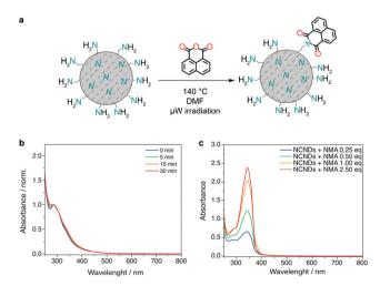
Fig. 2 Probing the imidization reaction. (a) Scheme for the model reaction with 1,8-naphthalic anhydride. (b) UV-vis spectra of CDs under different times of  $\mu$ W irradiation. (c) UV-vis spectra of CDs reacted with different amounts of 1,8-naphthalic anhydride for 30 min.
