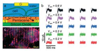
Fig. 15 Water-gated organic field effect transistors (WGOFET) neuronal transducer. (a) Schematic model of the device and interactions with adhering cells. (b) Drain current time traces recorded from a differentiated network after stimulation with various intensities. (c) Fluorescent microscopy image which indicates the formation of a functional neuronal network derived from murine stem cells on the transistor surface. 262
