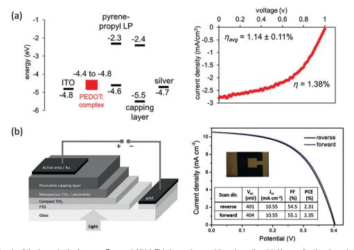
Fig. 8 (a) Energy levels of the layers in the (pyrene-O-propyl-NH<sub>3</sub>)<sub>2</sub>Pbl<sub>4</sub> layered perovskite solar cell and I-V curve for the champion device with 1.38% efficiency. (b) Schematic representation of the device configuration and photovoltaic performance of the champion device using Bn<sub>2</sub>Snl<sub>4</sub> pure 2D perovskite. Figures reproduced with permission from: (a) ref. 21. Copyright 2018, American Chemical Society; (b) ref. 55. Copyright 2019, Wiley-VCH.
