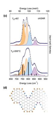
Fig. 3 Comparison between the HREEL spectra of N-doped (a) and pristine (c) chevron-type GNRs, obtained by deposition at  $T_D$  = 200 °C and at RT. The corresponding fitting components are shown as shaded curves, while calculated modes are displayed as black bars. The corresponding molecular schemes, showing the structure of the termini, are reported in (b) and (d), respectively. The top spectrum in (a) is also reported in the right panel of Fig. 1.
