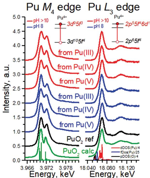
Fig. 3 Pu  $M_4$  and  $L_3$  HERFD experimental data. Data recorded for six  $\text{PuO}_2$  NPs samples and compared with a  $\text{PuO}_2$  reference and theoretical calculations, using AIM approximation (left) and FEFF code (right). The density of states is plotted at the bottom for clarity.
