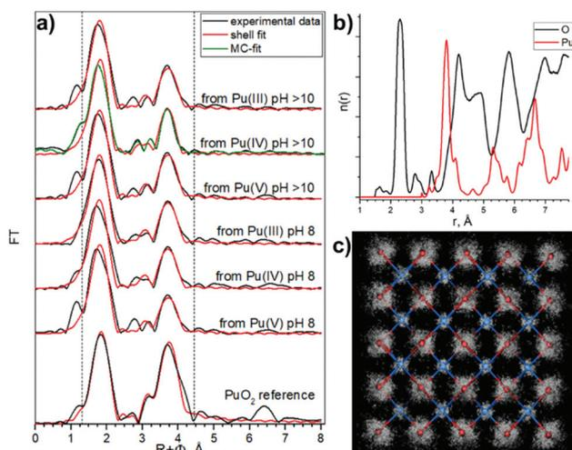
**Fig. 4** Pu L<sub>3</sub> EXAFS results. (a) Pu L<sub>3</sub> EXAFS spectra  $\chi(R)$  fit results, Fourier transform (FT) magnitude of experimental EXAFS data (black) and a one Pu–O, one Pu–Pu shell fit (red), Monte–Carlo simulations (green). The area of the shell fit in  $R$ -space is marked with two dashed lines, (b) MC simulation output: radial particle distribution function ( $n(r)$ ) for Pu–O and Pu–Pu, (c) 3D structural refinement based on bulk PuO<sub>2</sub> structure.
