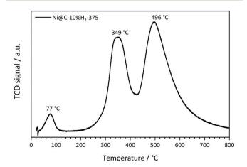
Fig. 11 Temperature-programmed reduction profile of Ni(BDC)(PNO) decomposed at 375 °C in 10%  $\rm H_2/He$ .
