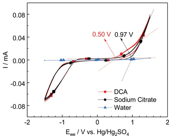
Fig. 2 Current vs. voltage response for sodium citrate ([sodium citrate]: 1.35 mM, [citric acid]: 1.15 mM),  $\text{DC}^{2-}$  ([DCA]: 2.5 mM, [NaOH]: 4 mM), and diluted HCl solution. Conditions: 25 °C, pH 4.9.
