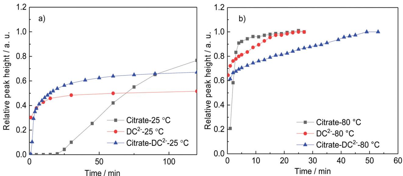
**Fig. 1** Comparison of the rate of formation of gold nanoparticles (represented by the relative height of the absorption peak) using sodium citrate or  $\text{DC}^{2-}$  as a reducing agent at a. 25 °C and b. 80 °C. Conditions:  $[\text{HAuCl}_4]$ : 0.25 mM, pH: 4.8–4.9, reducing agent: [sodium citrate]: 2.5 mM,  $[\text{DC}^{2-}]$ : 2.5 mM; or [sodium citrate] 2.5 mM +  $[\text{DC}^{2-}]$  2.5 mM, as in experiments A–F (Table 1).
