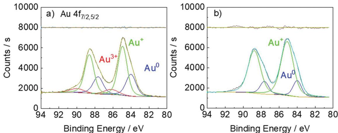
Fig. 6 XPS of a. [HAuCl<sub>4</sub>]: 0.25 mM, [DC<sup>2-</sup>]: 2.5 mM, sampling time: 5 min; b. [AuCl]: 0.25 mM, [DC<sup>2-</sup>]: 2.5 mM, sampling time: 15 min. Conditions: pH: 4.8, 25 °C.
