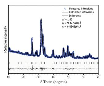
Fig. 2 Rietveld fit to cHAP powders XRD data. Experimental (O) and calculated (-) patterns are shown along with the difference curve (-) and (I) Bragg positions.
