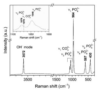
Fig. 3 Raman spectrum of cHAP powders calcined at 800  $^{\circ}$ C (inset: enlarged spectrum region of overlapping bands assigned to  $PO_4^{3-}$  and  $CO_3^{2-}$  modes).
