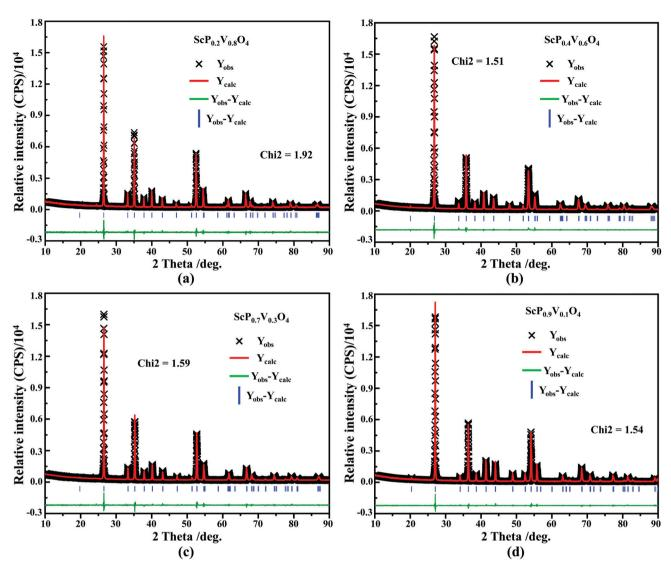
Fig. 3 Refined XRD patterns (–) of the typical samples of  $SCP_{0.2}V_{0.8}O_4$  (a),  $SCP_{0.4}V_{0.6}O_4$  (b),  $SCP_{0.7}V_{0.3}O_4$  (c), and  $SCP_{0.9}V_{0.1}O_4$  (d), where the Rietveld refining results (×), Bragg reflections (|) and the profile difference between observed and calculated values (–) are also given.
