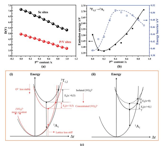
Fig. 7 (a) Calculated D values for the Sc (black) and P/V (red) sites; (b) variation of emission energy and energy barrier  $\Delta E_a$  in the obtained Sc( $P_x$ ,  $V_{1-x}$ )O<sub>4</sub> solid solutions; (c) single coordinate configurational diagrams based on the potential energy of the (VO<sub>4</sub>)<sup>3-</sup> luminescent unit.
