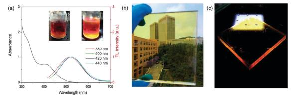
Fig. 12 (a) Absorption and PL spectra of C-dots dispersed in methanol solution. The excitation wavelength is 380-440 nm. Photographs of the LSC under ambient (b) and one sun (100 mW cm<sup>-2</sup>) illumination (c). Reproduced with permission from ref. 126. Copyright 2019 Elsevier.
