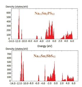
Density of states of Na<sub>11</sub>Sn<sub>2</sub>PS<sub>12</sub> and Na<sub>11</sub>Sn<sub>2</sub>SbS<sub>12</sub>.
