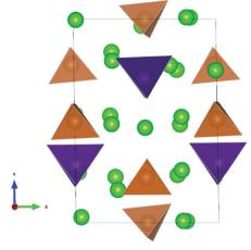
Fig. 3 The lowest energy configuration of Na<sub>10</sub>SnP<sub>2</sub>S<sub>12</sub>. Purple (brown) tetrahedra represent SnS<sub>4</sub> (PS<sub>4</sub>); green spheres indicate occupied Na sites.
