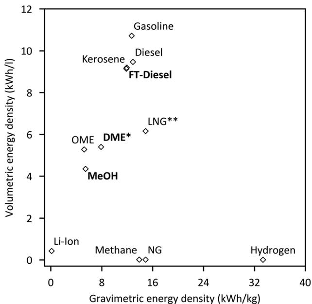
Fig. 1 Gravimetric and volumetric energy density of different fuels and Li-Ion batteries for comparison (\*at 10 bar; \*\*at  $-160\text{ }^{\circ}\text{C}$ ).<sup>13–15</sup>
