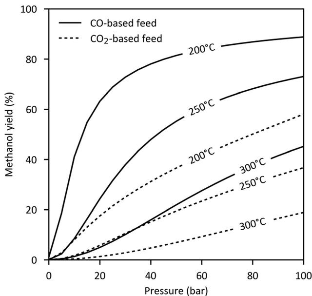
Fig. 4 Equilibrium conversion of CO- or CO<sub>2</sub>-based feed gas to methanol.
