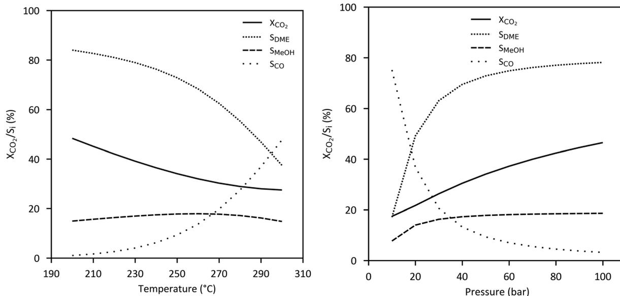
Fig. 13 Equilibrium conversion of CO<sub>2</sub> ( $= [\text{CO}_{2,\text{in}} - \text{CO}_{2,\text{out}}]/\text{CO}_{2,\text{in}}$ ) and selectivity of DME, methanol and CO ( $S_i = i/[\text{CO}_{2,\text{in}} - \text{CO}_{2,\text{out}}]$ , with  $i = 2 \times \text{DME}/\text{MeOH}/\text{CO}$ , based on amount of C-atoms) dependent on (a) temperature and (b) pressure ( $\text{H}_2 : \text{CO}_2 = 3 : 1$ , based on Aspen Plus Simulation).
