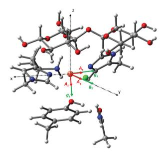
Fig. 5 Cartoon representation of the calculated relative orientation of the q (green) and  $A^{Cu}$  (red) principal components with respect to the molecular frame (black dotted vectors).
