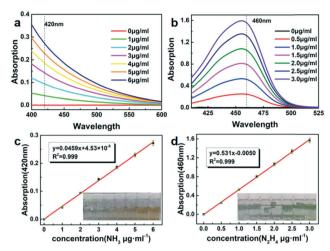
Fig. 5 (a) UV-vis curves of Nessler's reagent tests with NH<sub>4</sub><sup>+</sup> ions. (b) UV-vis curves of Watt and Chrisp method tests with hydrazine. (c) Calibration curve used for the estimation of NHz. (d) Calibration curve used for the estimation of hydrazine.
