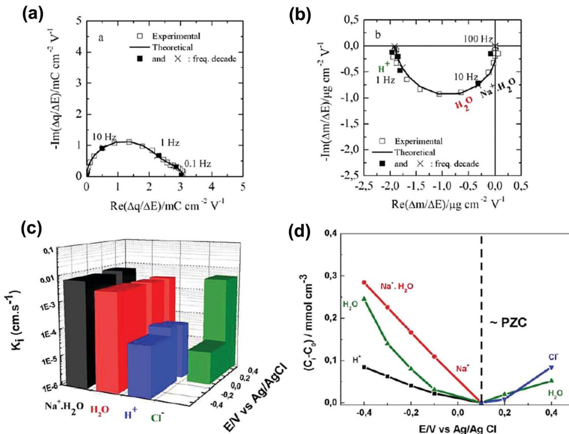
Fig. 8 (a) and (b) The transfer functions  $\frac{\Delta q}{\Delta E}(\omega)$  and  $\frac{\Delta m}{\Delta E}(\omega)$  at  $-0.4$  V vs. Ag/AgCl, respectively. (c) The kinetic parameters  $K_i$  ( $\text{cm} \cdot \text{s}^{-1}$ ) for each ion at different applied potentials. (d) Relative concentration variation of each ion in SWCNT based thin films as a function of potential in 0.5 M NaCl at pH = 7. Reproduced from ref. 173 with permission from Elsevier (copyright 2016).
