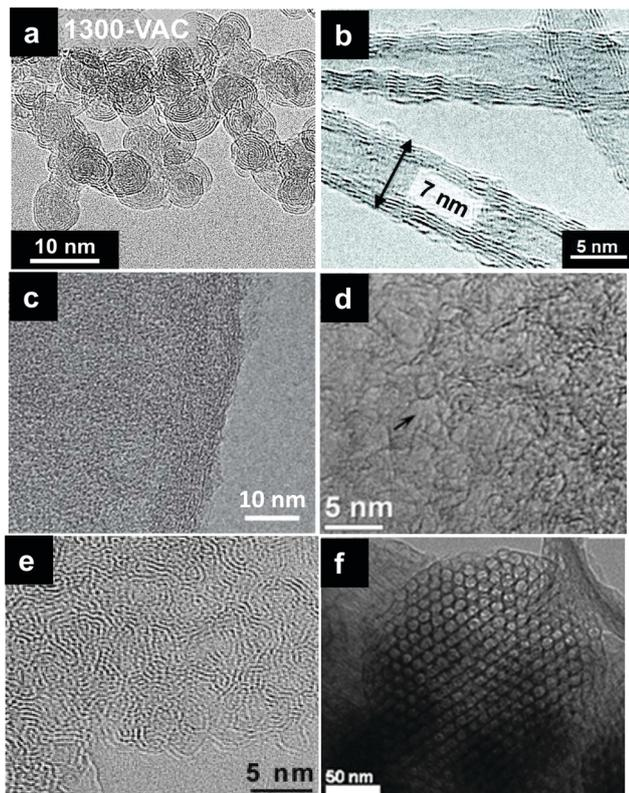
**Fig. 3** Transmission electron micrographs (TEM) of various carbons with several dimensionalities for EDLCs: (a) OLCs,<sup>94</sup> (b) CNTs,<sup>76</sup> (c) graphene,<sup>92</sup> (d) ACs,<sup>95</sup> (e) CDCs,<sup>65</sup> and (f) TCs,<sup>96</sup> with permission from Elsevier (copyright 2015), 2011 American Chemical Society, Springer Nature (copyright 2014), Elsevier (copyright 2019), Elsevier (copyright 2006), and Royal Society of Chemistry (copyright 2009), respectively.
