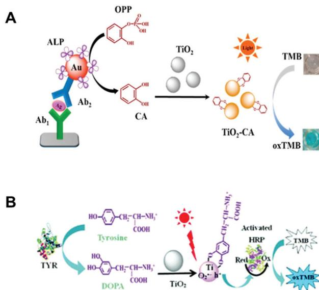
Fig. 7 (A) Proposed immunodetection process for mouse IgG by coupling the *in situ*-generated photo-responsive nanozyme of CA- $\text{TiO}_2$ . (B) Schematic illustration of the colorimetric sensing mechanism for TYR based on the photoactive sensor. (A) Reproduced from ref. 79 with permission from the American Chemical Society, copyright 2015. (B) Reproduced from ref. 80 with permission from the Royal Society of Chemistry, copyright 2017.
