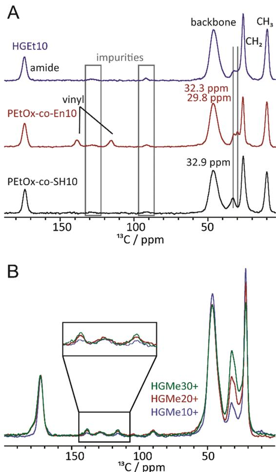
Fig. 6 (A)  $^1\text{H}$ - $^{13}\text{C}$  CP/MAS solid-state NMR spectra of the cross-linked hydrogel HGET10 (blue) as well as the two precursor polymers with thiol and vinyl units and (B)  $^{13}\text{C}$  CP/MAS solid-state NMR spectra of HGMe10+, HGMe20+ and HGMe30+. All experiments were recorded at 14.1 T and 12.5 kHz MAS. For the CP/MAS experiments, a contact time of 2 ms was used.
