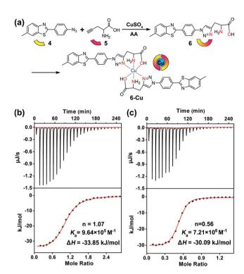
Fig. 2 Cu-chelating properties of 6. (a) Scheme of the synthesis of the bifunctional compound 6. (b and c), ITC data of  $CuCl_2$  binding to Aβ40 and compound 6, respectively. The bottom panels show the fitting results. Details are described in the Experimental section.
